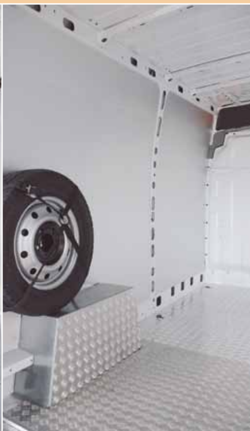
Rivestimento interno in alluminio 12/10 Internal wall's cover aluminium 12/10 Innenverkleidung aus Alu 12/10
